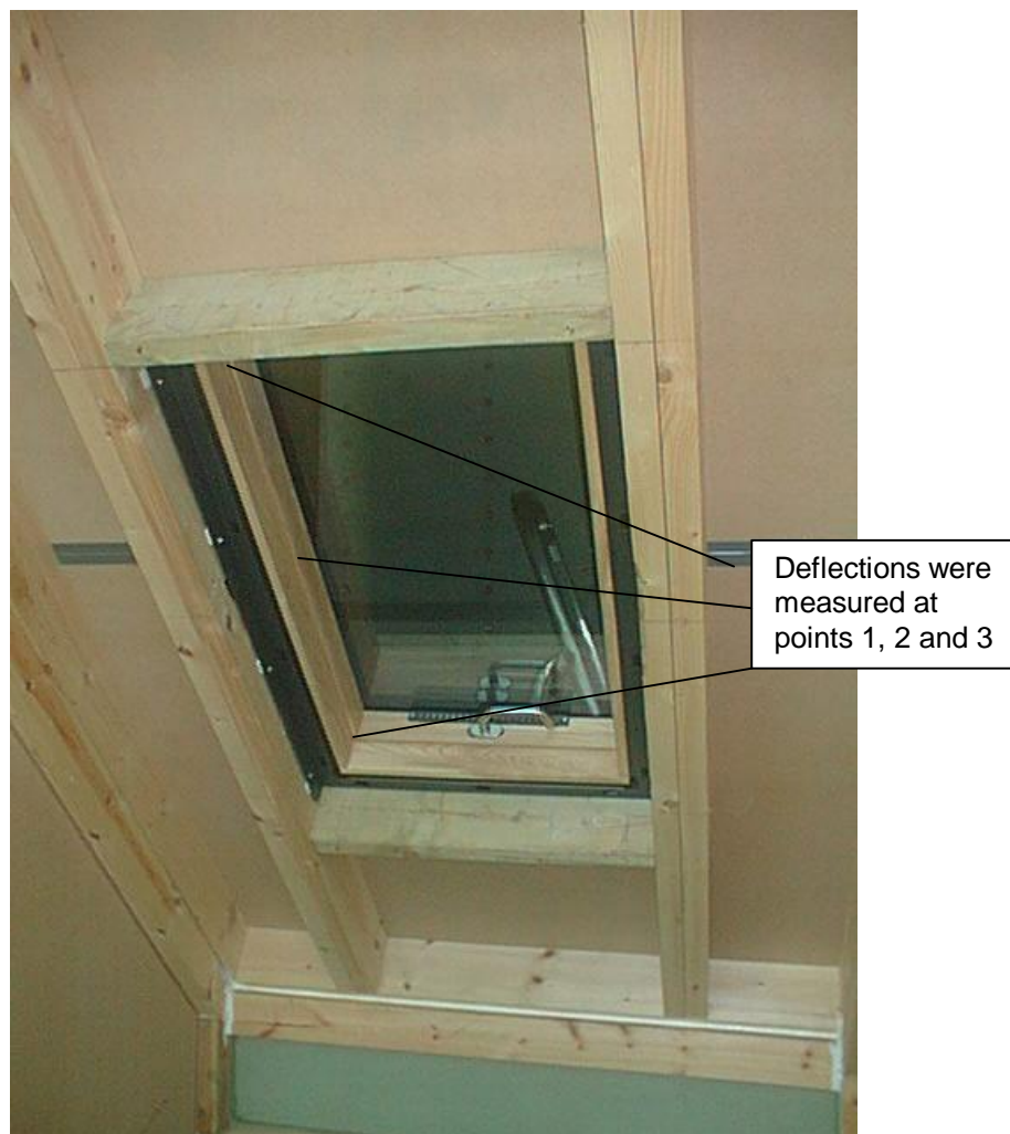
Figure A2. The test specimen installed in the BRE 'G' Weathertightness test rig showing points where deflections were measured.
