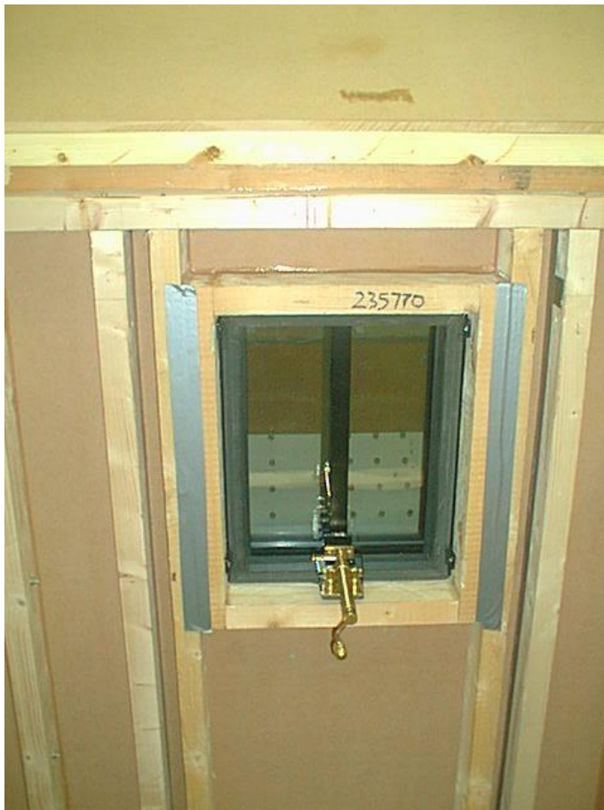
Figure A2. The test specimen in place on the weathertightness test rig
